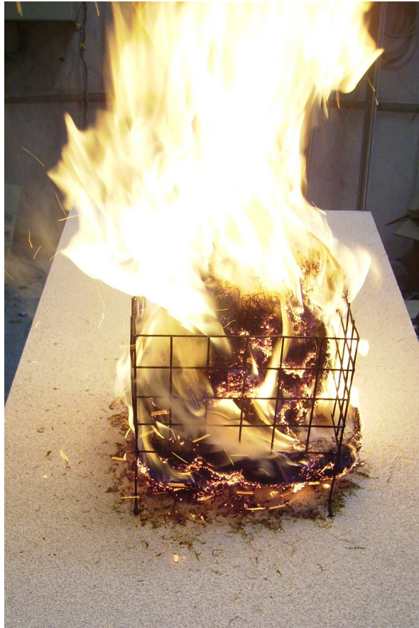
Appearance of the sample during the External Fire test Test 1: method with burning torches in accordance with ENV 1187:2003
