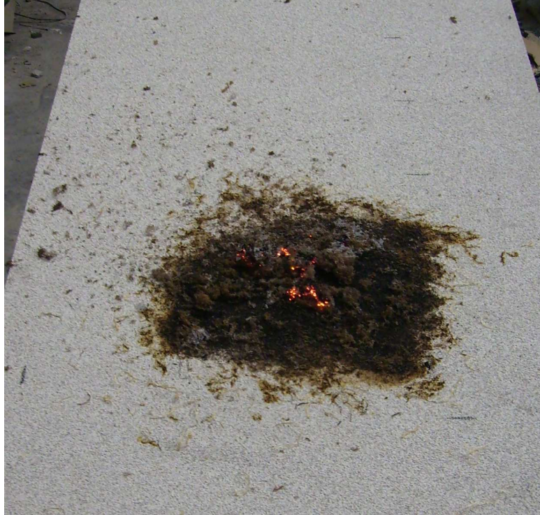
Appearance of the sample after the External Fire test. Test 1: method with burning torches in accordance with ENV 1187:2003
