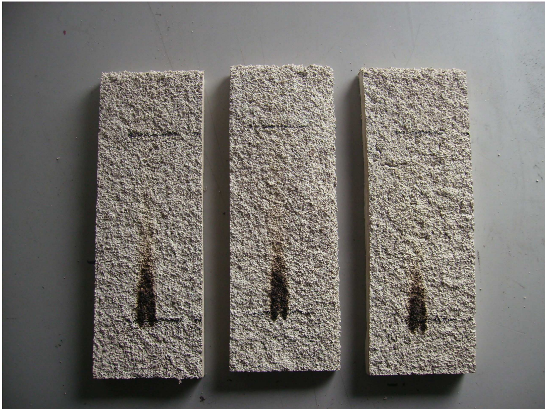
Appearance of the sample after the ignitability test in accordance with UNE-EN ISO 11925-2:2002
