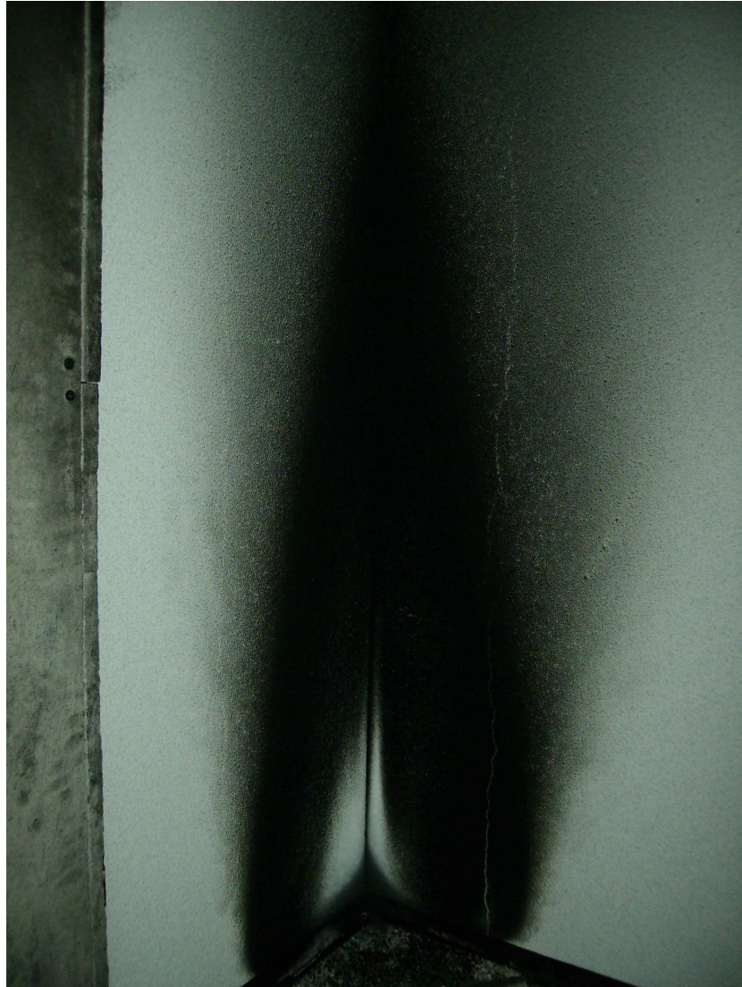
Appearance of the sample after the SBI test in accordance with UNE-EN 13823:2002
